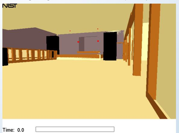
Computer simulation of The Station fire had sprinklers been installed
